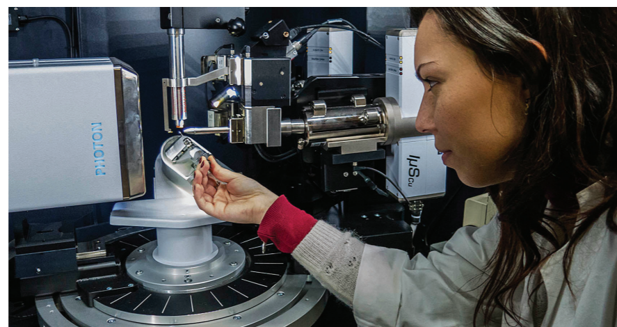
KAPPA four-circle goniometer in a microfocus X-ray diffractometer and photon counter CMOS detector
